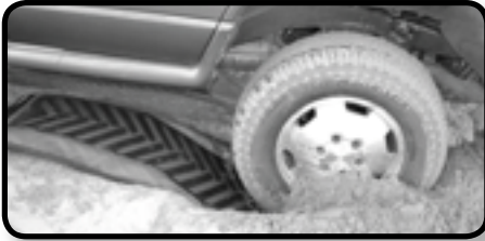
Place the deflated Pillowtrack (as flat as possible) and push it towards the wheel.
