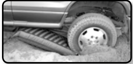
Inflate the Pillowtrack until it looks full and feels firm. Do not over inflate – 3-5 PSI is sufficient.
