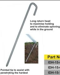
Fed-up with bent or rusted tent pegs? 304 STAINLESS STEEL will eliminate your rust problem forever and it's tough tensile strength (800MPa\*) will significantly reduce your bending problem compared with conventional mild steel tent pegs. (\*Mild Steel 420MPa)
