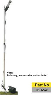
The *Light or Shower Pole* is made up of 3 sections of high grade aluminium tube. It has a cam-loc mechanism at each section allowing telescopic extension from 1.0m up to 2.3m. There is an adaptor sleeve at the base for connection to the *Ground Peg* or *Battery Plate*. The threaded spigot at the top is designed to secure the optional *Shower Arm* or *Wire Light Holder*.
