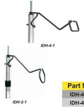
This brilliant design allows you to hang your rectangular or round 12v portable light just about anywhere, utilising the free standing *Light Pole* or any 22mm diameter tent pole. Because of it's positive location over the spigot, your light will not come crashing down if knocked or in strong winds. It is made from 5mm steel wire and is nylon coated for added durability.
