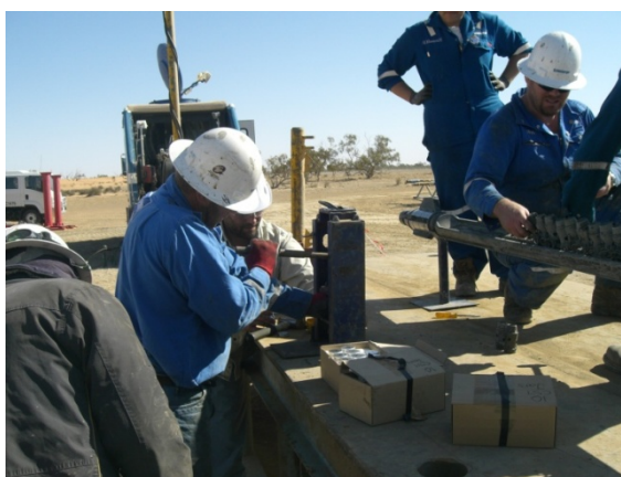
Retrieving side wall cores from Wakefield 1, Cooper Basin
