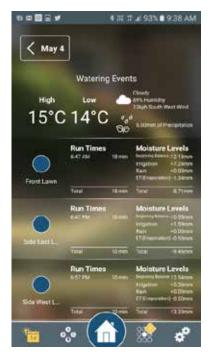
Result of Irrigation showing: Starting moisture level, irrigation, rain fall, evaporation equalling net moisture in root zone
