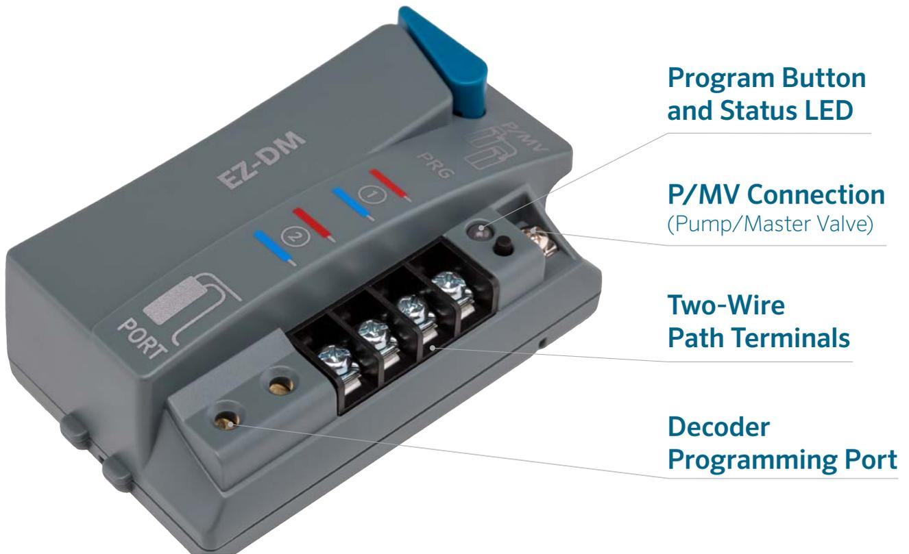
Plug in the EZ-DM two-wire output module to enable up to 54 stations of irrigation, plus a master valve, on a single pair of wires. Then simply place EZ Decoders at each valve!
