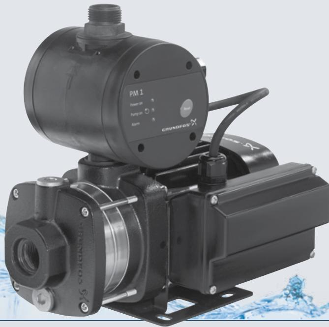
The Grundfos CMBasic is a compact booster pump designed for domestic and light industrial use. The booster unit consists of a Grundfos CM cast iron pump and PM1 pressure manager. The pressure manager allows the pump to start and stop automatically according to demand and protects the pump from dry running.
