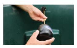
3. Attach float to threaded end of lever.
