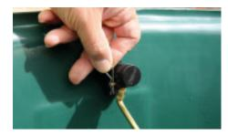
6. Adjust the lever arm and then refit. Once the correct lever arm angle is achieved ensure the pivot pin is secured with the R-pin.
