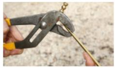
5. Using a pair of multi-grips or equivalent the lever can then be bent to the necessary angle.
