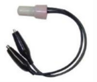
Valve locators are devices which alternate the on and off selection of the circuit at a medium frequency creating an audible rattle sound from the movement of the electric coils magnetically drawn shaft and seat. This can usually be heard through several hundred millimetres of earth.
