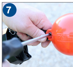
7 Using a Phillips head screwdriver unscrew Float
