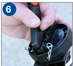
6 Reinstall float arm using pivot pin and replace the R-Pin
