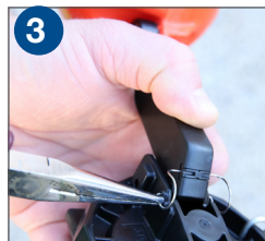
8 Unclip damper spring from cap
