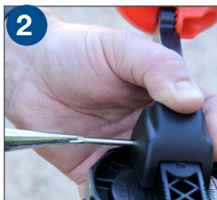
7 Remove pivot pin, dispose of spring cover
