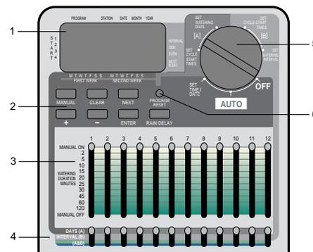
FIGURE 1: Features of the Controller
