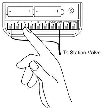
**FIGURE 24: Connecting Valve Wires**
