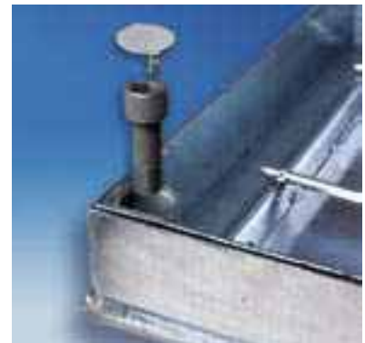
Four high tensile steel M16 recessed socketed locking bolts per cover with plastic cap to protect from dirt ingress. Lifting bosses use standard AS 3996 lifting keys.
