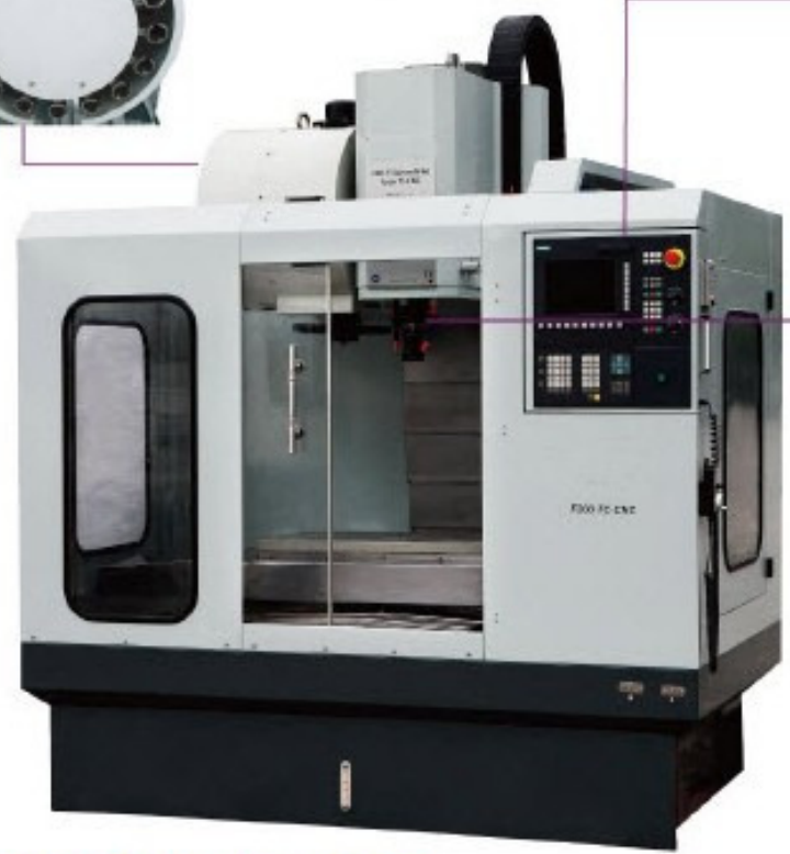
Automatic Tool Change System With 16 Tool Magazine.
