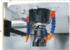
Automatic timer adjustable Lubrication System.
