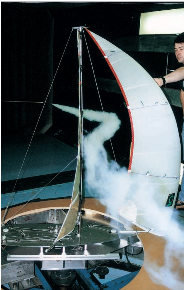
Smoke shows the air flow over the sail. When trim or sail shape changes, the pattern of the smoke gives immediate feedback—the less “swirling,” the better.
