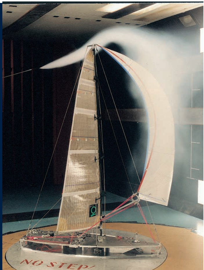
Smoke shows the air flow over the sail. When trim or sail shape changes, the pattern of the smoke gives immediate feedback—the less “swirling,” the better.
