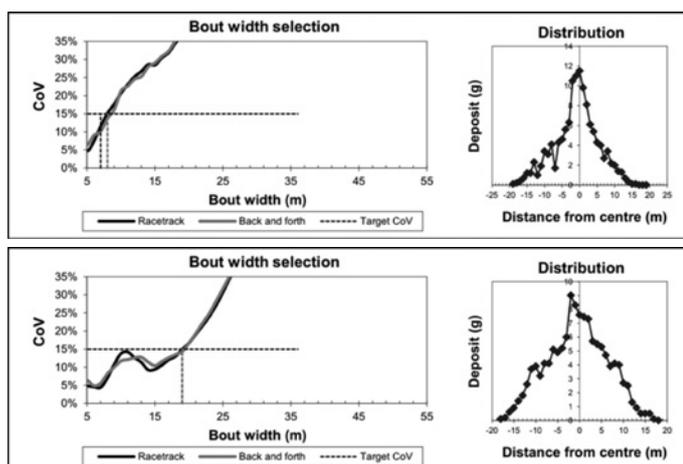
**Figure 1:** 15% coefficient of variation (CoV) is the critical level indicating how wide a spreader is effectively distributing fertiliser. In this example, blades were replaced on an older machine and a new 'V' fitted to better direct the fertiliser into the middle of the spinners. The spread width for this spreader increased from 7m to 19m.
