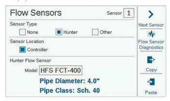
Select the sensor input number to be setup (1-6). The controller has 3 Flow Sensor inputs built in, but 3 more can be added with the A2C-F3 Flow Expansion module.
