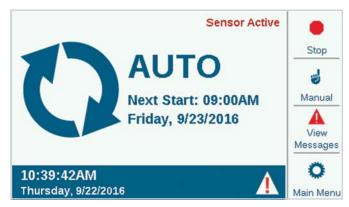
If Solar Sync is installed and enabled (Devices menu), the Solar Sync symbol shows the current adjustment percentage in the lower right of the border.
