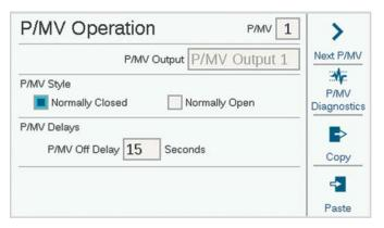
All P/MV outputs are set to Normally Closed operation, but they can be changed to Normally Open functions in the Devices menu. See P/MV Operation section on page 18.
