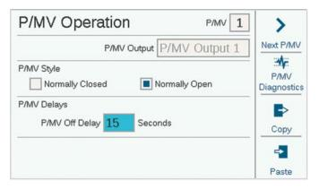
Normally Open may also be selected, and is discussed further in the Flow Operations section. Normally Open is not a station level setting. The valve is always open until a problem is detected at the Flow Zone, or MainSafe level, when the controller activates the normally-open P/MV to shut the water off.
