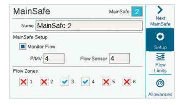
MainSafe zones generally require their own flow sensor, and their own Master Valve. Often these are Normally Open Master Valves, which only close in the event of an alarm.
