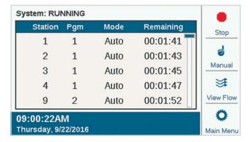
The soft keys normally show Stop, Manual, View Flow (shows current flow if a flow sensor is installed and enabled), and Main Menu. Stop and Manual are described in the Basic Programming section. View Flow is described in detail in the Flow Operations section.
