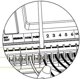
Small Hole-for running 5 or 7 strand wire straight into the box
