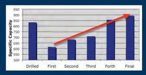
The Quinns water supply well was cleaned with BoreSaver Ultra C using the surge/brush method. Due to the extreme clogging four cleaning phases were used. Recovery exceeded the original drilled pump test.
