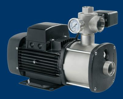
The CM-PS is a compact booster solution designed for domestic and light industrial use. The booster unit consists of a robust CM pump, 5-way valve and a pressure switch. To complete the booster system a pressure tank must be fitted. The pressure switch and pressure tank ensure a convenient water supply with a minimum start/stop frequency.
