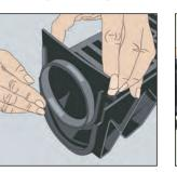
2. Insert End Cap or End Outlet • Join Reln Storm Drain System. Joins and End Caps may be sealed with silicone. Use Reln End Cap at highest point of Reln Storm Drain Channel. Connect the low end of the Storm Drain Channel to a Rainwater Pit, or, using 90mm PVC pipe use built in Bottom Outlet, or fit an End Outlet to allow water to clear. Lay Storm Drain Channel out with 90° Corner Piece or Tee Piece connected and End Cap fitted prior to concreting.
